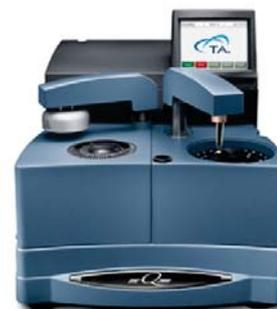
DSC is used to examine the thermal transitions in a polymeric material (e.g. melting point, T<sub>g</sub> and crystallization).
