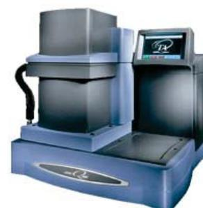
DMTA is a technique used to analyse the viscoelastic behaviour of a material as a function of temperature or frequency. The DMTA measurement results are used for determining thermal transitions such as the glass transition temperature (T<sub>g</sub>). A DMTA diagram shows the stiffness (storage and loss modulus) as a function of temperature.
