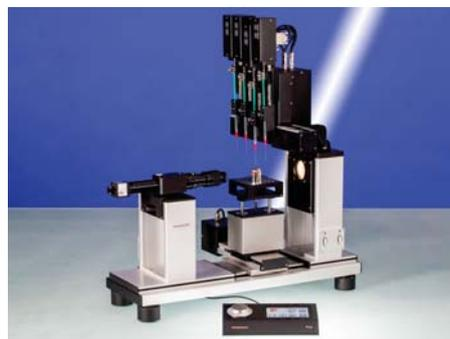
Contact angle measurements can be done on flat surfaces to determine its hydrophobic or hydrophilic behavior. A total of 10 drops will be placed on the to be measured surface which are then imaged by a camera. Via the software the contact angle at the left and right side is then calculated, and gives an average over the 10 droplets. With contact angle measurements a variation of +/- 3° in between measurements is within the tolerance limits.
