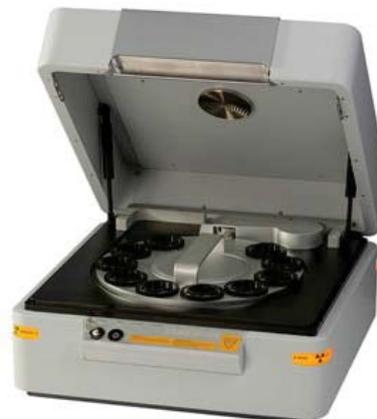
X-ray fluorescence (XRF) is an analytical technique that can be used to determine the chemical composition of a wide variety of sample types including solids, liquids, slurries and loose powders. X-ray fluorescence is also used to determine the thickness and composition of layers and coatings. It can analyze elements from beryllium (Be) to uranium (U) in concentration ranges from ppm to 100% levels.
