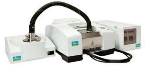
The two techniques of TGA and IR spectroscopy can be combined to obtain additional information on a material.
