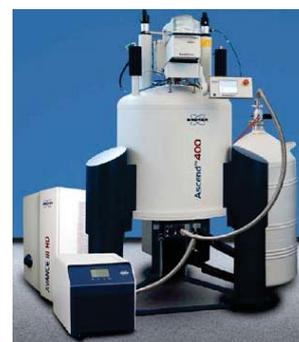
Solution NMR spectroscopy is a non-destructive analytical technique used for identification and quantification of a sample. The technique gives detailed structural information about the structure of organic compounds, including polymers. Chemical transformations can conveniently be monitored using NMR spectroscopy as well.
