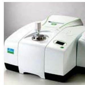
IR spectroscopy is used to record an IR spectrum of a material that is unique to that type of material, in other words a fingerprint of the material.
