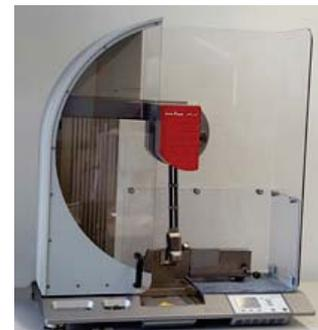
The impact test is a standardised method for analysing the toughness or brittle-fracture sensitivity of a material. Measurements are carried out with a Zwick/Roell HIT5.5P impact tester equipped with all hammers suitable for use with plastics. Measurements can be carried out at room temperature as per IZOD (ISO 180) or Charpy (ISO 179). The specimens can be notched with the help of a standardised notch-cutting machine.
