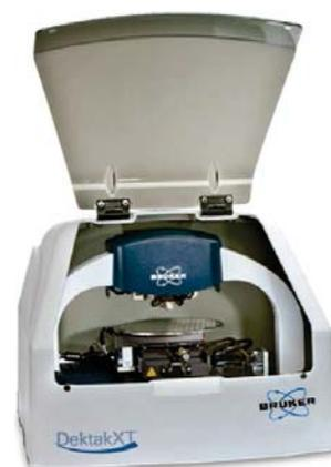
Surface profilers are commonly used for measuring thin film thickness, and surface roughness and form in applications ranging from educational research verification to semiconductor process control. The tip of a stylus gently moves over the surface of a flat surface in one line, leading to a two-dimensional surface profile. When multiple lines next to each other are combined a three-dimensional plot can be derived and analysed.
