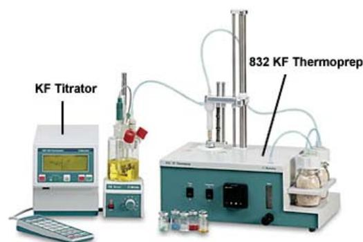
Karl Fischer titration is a technique used for measuring the water content of a sample. The sample can be an organic solvent or a solid. Measurements are carried out with a Metrohm 831 KF Coulometer in combination with a Thermoprep 832 oven. Solid samples can be measured over a temperature range of 30 to 250  $^{\circ}\text{C}$ . Karl Fischer titration allows accurate measurement of water content from ppb-level to 100%. Being a selective method, it reacts to water only.
