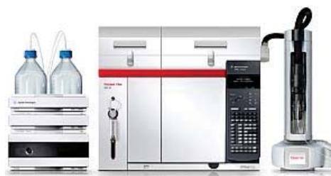
HT-GPC or HT-SEC is employed to determine of the average molecular weight ( $M_n$  and  $M_w$ ) and the polydispersity index ( $M_w/M_n$ ) of highly crystalline polymers which show low solubilities in common organic solvents at ambient temperature.
