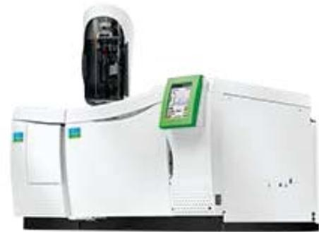
Gas Chromatography combined with Mass Spectrometry is a way to identify or quantify (semi) volatile compounds. The sample is injected into the GC-MS and separated based on boiling point and affinity with the column. The separated components are then detected with a Mass Spectrometer resulting in a mass spectrum unique for a material. The obtained mass spectra are run through the NIST database to identify the detected components.
