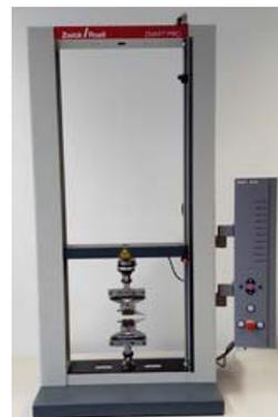
A tensile tester is used to determine the elongation, compression and bending characteristics of a material.
