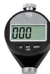
The Shore Hardness scale indicates the resistance of a material to indentation. A Shore durometer has a needle on a spring which is placed against the material and pressure is applied. Once the durometer is pressed firmly against the material and the needle has penetrated as far as it can go, the corresponding shore hardness can be read from the display.
