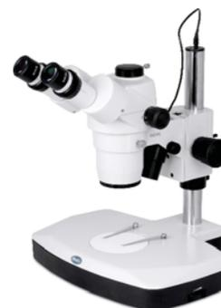
A stereo microscope is a microscope with two objective lenses and two eyepieces, which makes it possible to visualise a sample in 3D. Measurements are carried out with a Motic Stereo SMZ-168T-LED microscope with a magnification range of 7.5x to 50x and the option to save the images.
