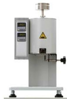
The MFI is a measure of the flow rate of a polymer melt (expressed in grams per 10 minutes) at a standard temperature and a standard load, in conformity with ISO Standard 1133.
