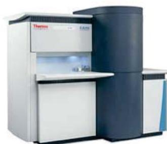
XPS analysis is a surface-sensitive quantitative spectroscopic technique that typically measures the top 0-10 nm of a sample surface. Elements from Lithium (Li) upwards in the periodic table can be measured.
